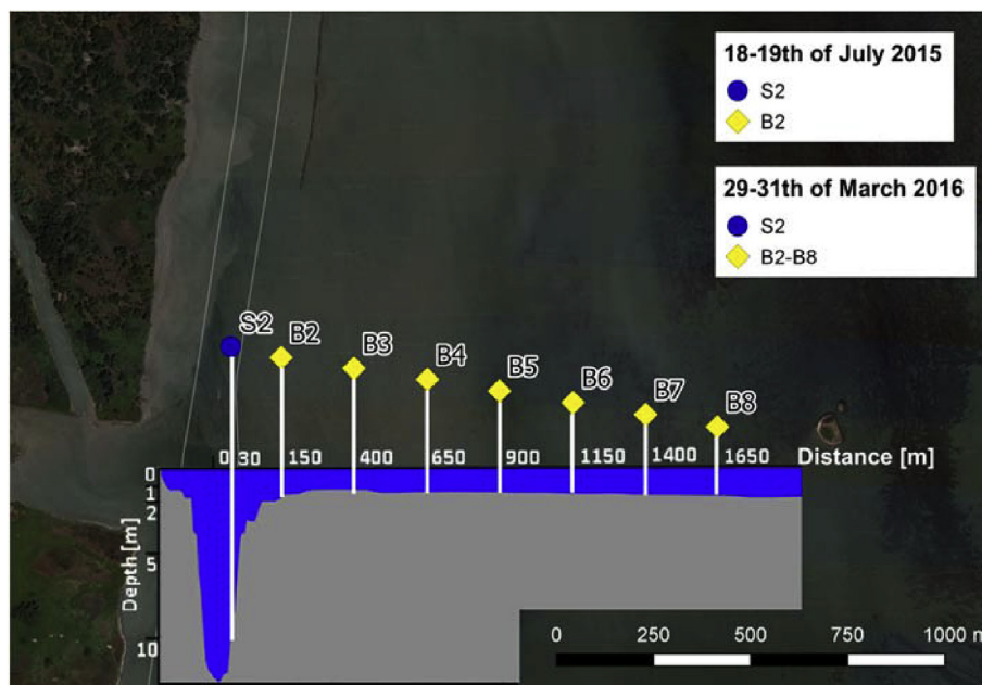
Fig. 4. Location of in situ instruments used for the measurements during the field campaigns in the MM channel and in the nearby tidal flat. The 18 th –19 th of July 2015, blue dot represents the S4 instrument, located in S2 station at the bottom of the border of the channel, and the yellow diamond in B2 represents the pressure probe on the tidal flat; the 29 th –31 st of March 2016, yellow diamonds represent pressure sensors in B2–B8 from the channel to the inner tidal flat, with an average spacing of 250 m. In B2 and B4 also the S4 instruments were deployed. The corresponding bathymetric profile is superimposed at bottom. (For interpretation of the references to colour in this figure legend, the reader is referred to the Web version of this article.)
