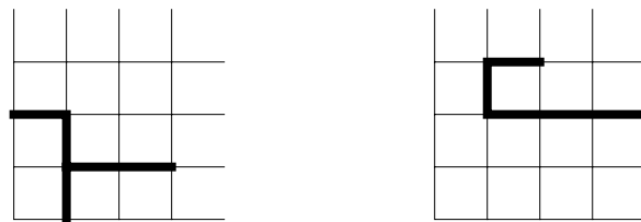
Figure 13.6: Two examples of bond clusters. The occupied bonds are shown as bold lines.
