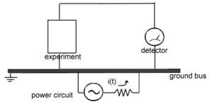
Cures for resistive coupling include: Grounding everything to the same physical point Using ground bus with lower resistance Remove sources of large currents from ground wires used for small signals
