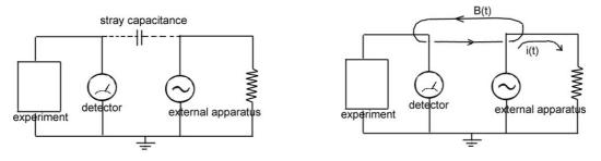
A possible cure is the reduction of the area of the pick-up loop by using twisted pairs or coaxial cables.
