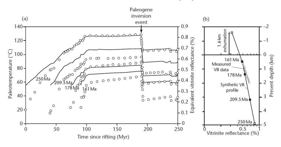
Paleotemperature and equivalent vitrinite reflectance versus time for four different horizons in a well in the extensional Irish Sea Basin ( $\beta$  = 1.5 at 250 Ma) with internal heat generation (A = 9.6 × 10<sup>-10</sup> W kg<sup>-1</sup>;  $h_r$  = 10 km) and variable thermal conductivity.
