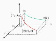
$$\begin{split} \varphi(\cdot,t_0,x_0,u(\cdot)) & \text{ state movement} \\ \varphi(t,t_0,x_0,u(\cdot)), & t \geq t_0 & \text{ state trajectory} \\ \eta(\cdot,\varphi(\cdot,t_0,x_0,u(\cdot))) & \text{ output movement} \\ \eta(t,\varphi(t,t_0,x_0,u(\cdot))), & t \geq t_0 \\ & \text{ output trajectory} \end{split}$$
