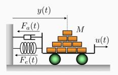
$$\begin{cases} u(t), t \in [t_0, t_1] \\ y(t_0) \\ \dot{y}(t_0) \end{cases} \implies y(t), t \in [t_0, t_1]$$
