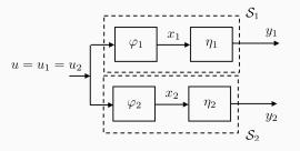
$$S = \{T = T_1 = T_2, U = U_1 = U_2, \Omega = \Omega_1 = \Omega_2, X = X_1 \times X_2, Y = Y_1 \times Y_2, \\ \Gamma = \Gamma_1 \times \Gamma_2 \}$$
