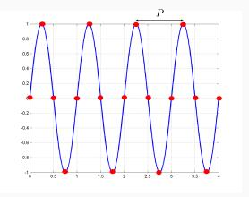
Reducing the sampling period (i.e. increasing the sampling frequency) the ambiguity disappears: no more frequency fold-over effect.
