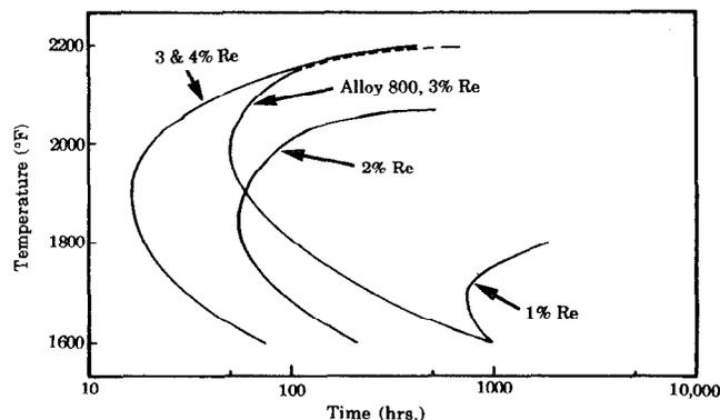
Figure 1. Comparison of TTT curve for formation of TCP phases in Alloy 800 with those of alloys 240 through 243<sup>(1)</sup>.
