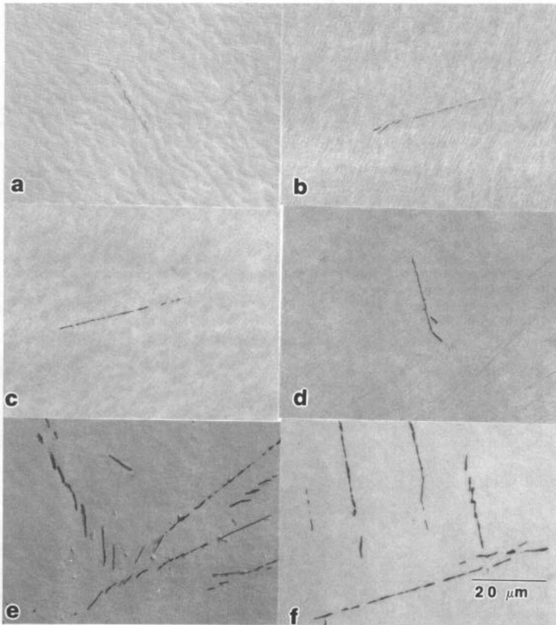
**Figure 2.** Optical micrographs showing the morphological development of the TCP phases at 2000°F a) 35 hrs., b) 50 hrs., c) 75 hrs., d) 100 hrs., e) 500 hrs., and f) 1000 hrs.
