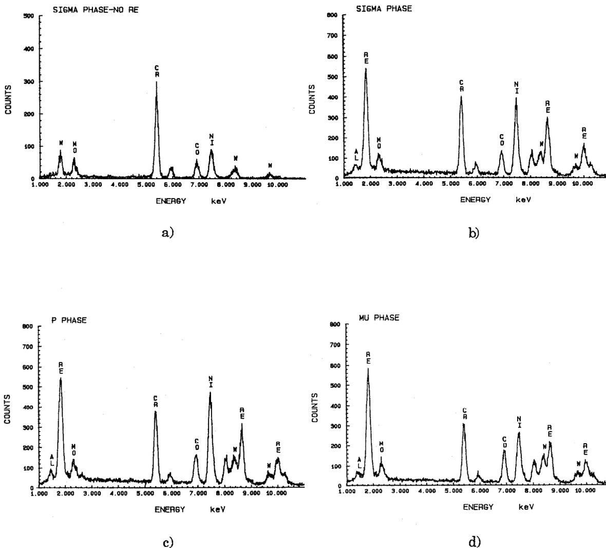
Figure 6. EDS spectra from TCP phases (a) Sigma phase in an alloy not containing Re, (b) sigma, (c) P, and (d) mu phase in an alloy containing Re.
