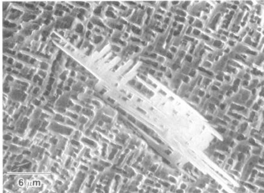
Figure 5a. SEM micrograph of TCP precipitate after 75 hrs. at 2000°F.
