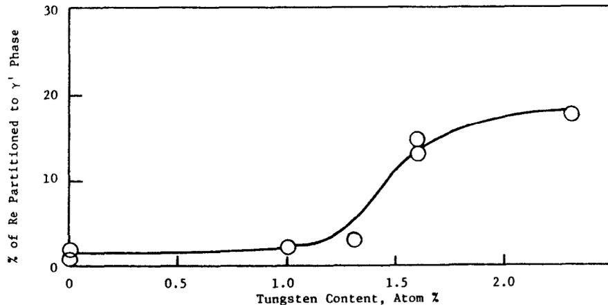
Figure 7. Plot showing synergistic effects of W and Re on gamma/gamma prime partitioning of Re.
