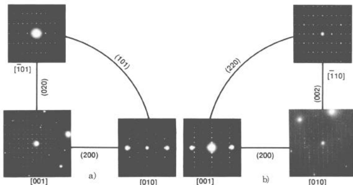
**Figure 3.** Selected area diffraction patterns from a) sigma precipitate, b) P precipitate in Alloy 800.
