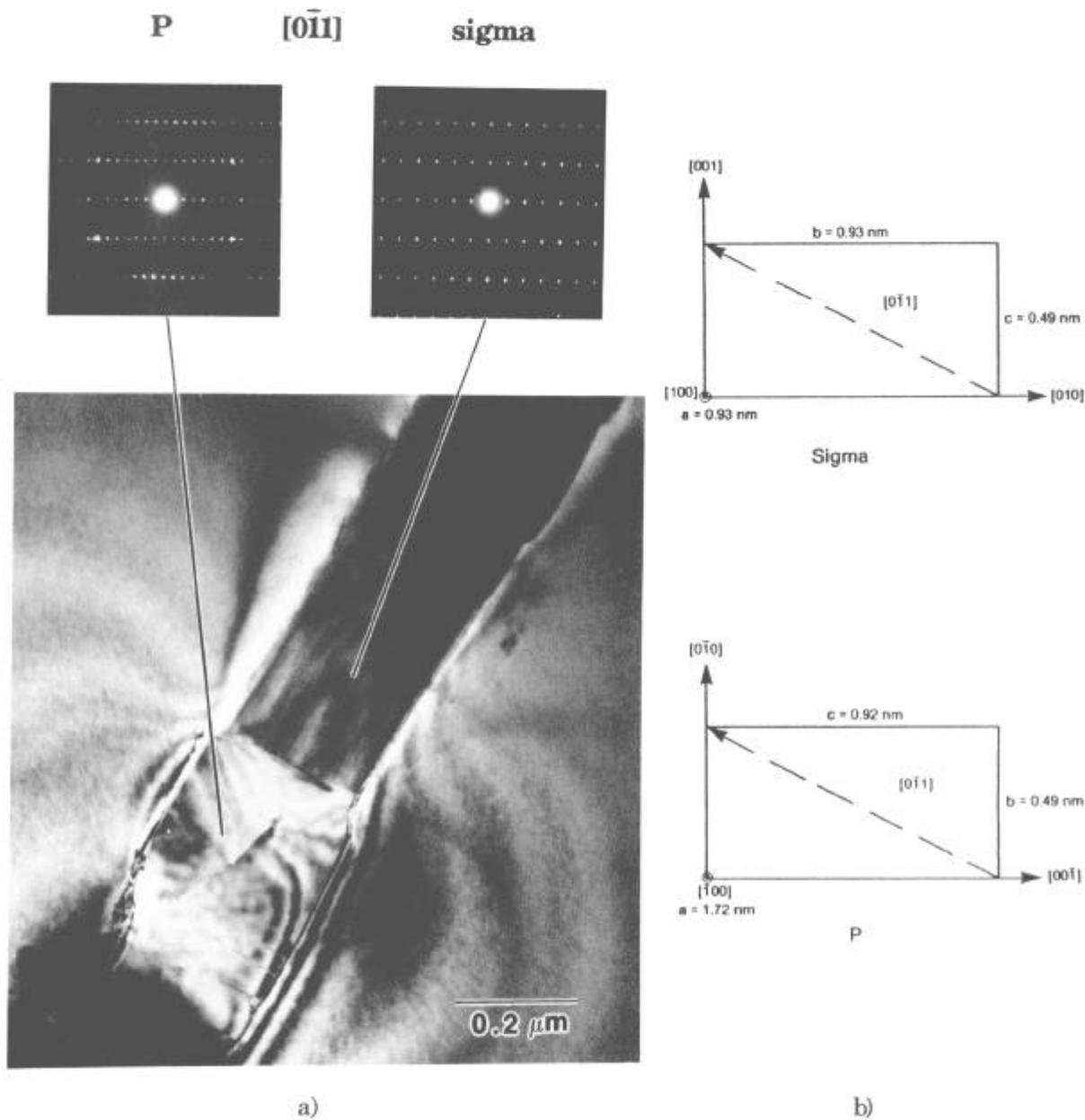
Figure 4. a) TCP precipitate consisting of P and sigma sections.
