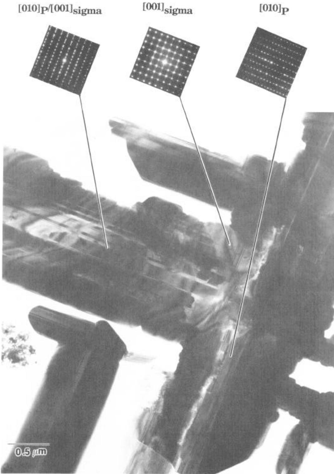
Figure 5b. TEM micrograph of extracted TCP precipitate after 75 hrs. at 2000°F. Note the crystallographic relationships between the various segments of the precipitate.
