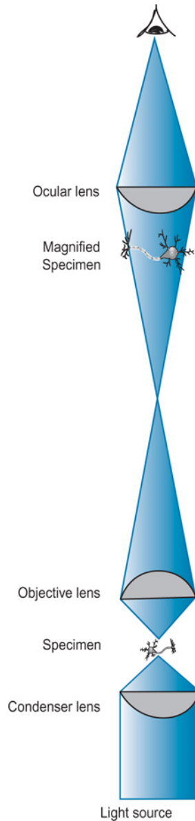
FIGURE 5.5 Compound microscopes use multiple lenses to magnify a specimen. A condenser lens focuses light onto a specimen, which then transmits (or reflects) light through the objective and ocular lenses that magnify the image that reaches the eye.
