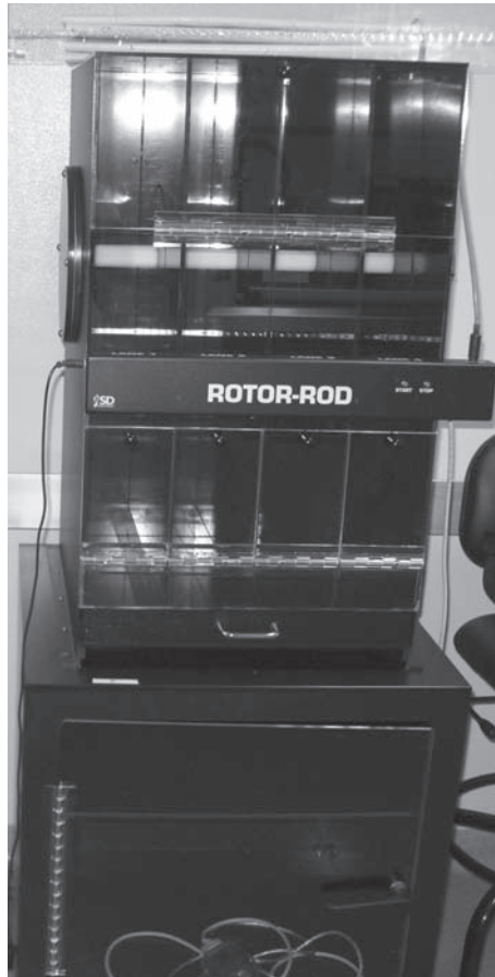
FIGURE 2.3 A rotarod tests balance and motor coordination. Multiple animals can be tested at one time with a device that has individual lanes to record each animal's latency to fall. (Courtesy of the Stanford Behavioral and Functional Neuroscience Laboratory.)
