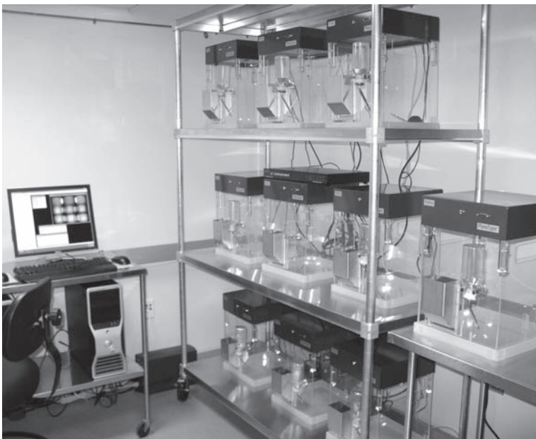
FIGURE 2.1 Locomotor activity can be monitored in a specially designed home cage. (Courtesy of the Stanford Behavioral and Functional Neuroscience Laboratory.)
