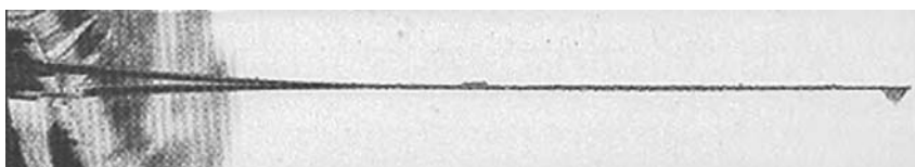
Fig. F2.3 The cantilever is the main element of an AFM. For biological applications, cantilevers are made of silicon nitride. The example shown is 200 \mu\text{m} thick and has a force constant of approximately 0.1 \text{ N m}^{-1} . Thus a measurable deflection is induced by forces of a few piconewtons. (Engel et al. , 1999.)
