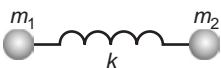
Fig. A3.11 Two masses connected by a spring of force constant, k .
