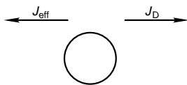
Fig. D5.4 Steady-state measurement in which fluxes J_{\text{eff}} and J_D are balanced.
