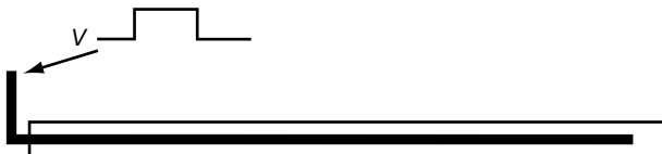
Fig. 16.4. The axial wire distributes an applied voltage ( V ) uniformly through an axon.
