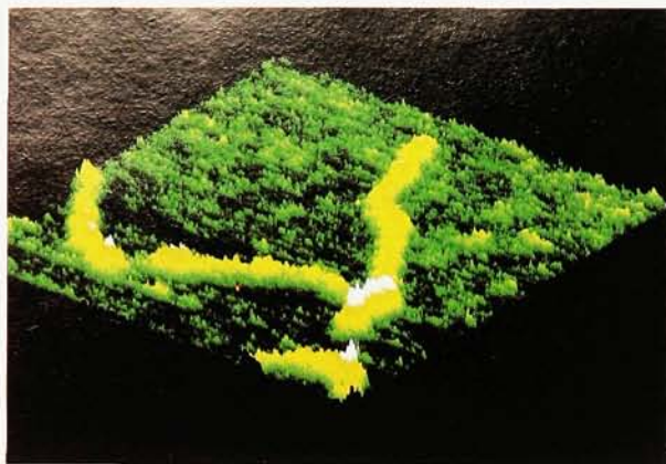
THREE CRO DIMER MOLECULES, each bound to its site at the O_R region in the DNA of bacteriophage \lambda . The dimers appear as three small light domes at the kink in the strand. The image was obtained in air using a tip produced by electron-beam deposition. The strand is about 200 nanometers long. (From ref. 9.) FIGURE 3
