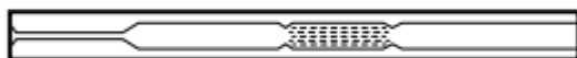
Figure 4: Example of Thermo Scientific Splitless FocusLiners 5 x 105 mm, note the different positions of the quartz wool packing
