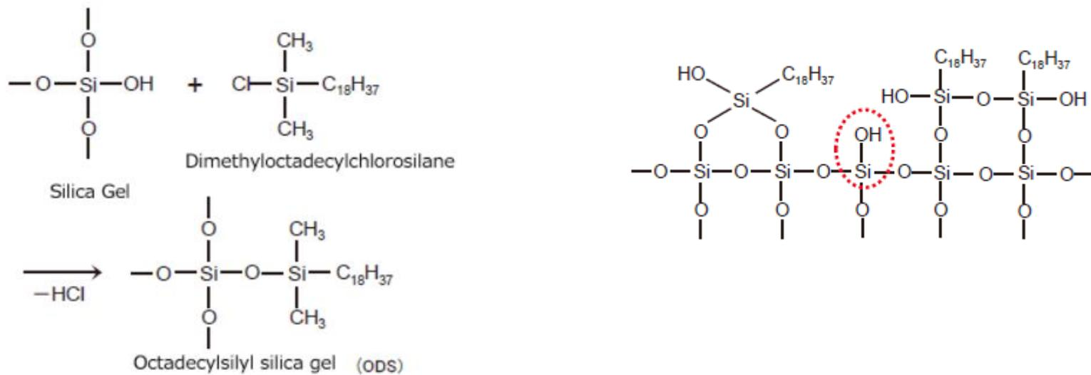
Fig. 2 Example Method of Preparing ODS
