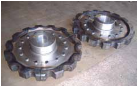
Ruota a segmenti Z=15 Segment wheels Z=15 Segmentkettenrollen Z=15
