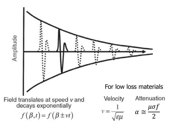
EM fields propagate as spatially damped waves when electrical losses are small. The signal amplitude decays exponentially in the direction of field translation while the field shape remains invariant. UD4a
