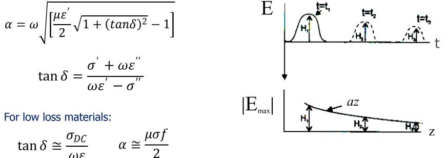
$\alpha$  is often referred as **INTRINSIC ATTENUATION** since it depends by EM medium parameters. The main physical parameter controlling the attenuation is the electrical conductivity  $\sigma$ , which varies by several order of magnitude. A minor effect is related to the dielectrical conductivity (polarization)  $\rightarrow \varepsilon$  varies by just two order of magnitude.
