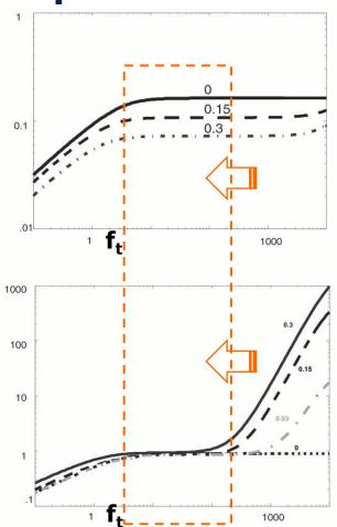
For real material containing varying water contents some dispersion can occur even within the **GPR plateaux**.
