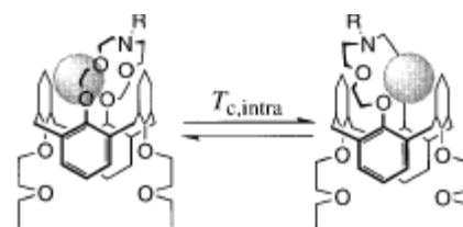
Figure 5. Schematic representation of a rope-jumping motion in the 1-Ag + complex.
