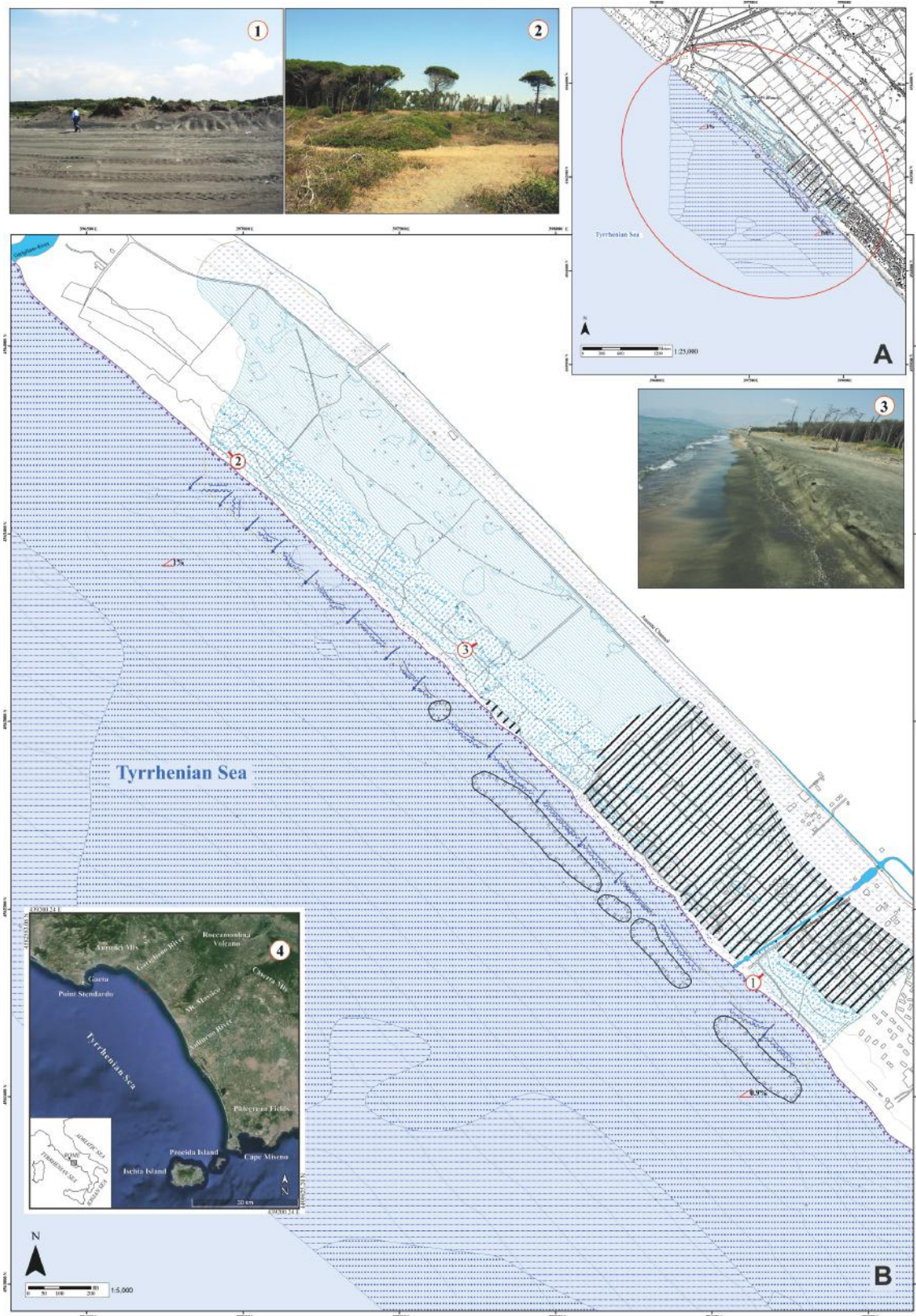
FIG. 10 - Geomorphologic maps of the SE of the Garigliano River Mouth (A, B): (1) anthropogenic remodeling of the beach due to cleaning and widening by mechanical vehicles; (2) blowout in the coastal dune modeled by wave erosion and airflow over the crest; (3) erosion scarp due to coastline retreat and consequent inland migration of beach-dune system; (4) coastal physiography of the Gulf of Gaeta. Circle in A indicates the location of the study area (B). See fig. 3 for legend.
