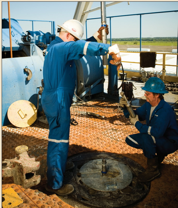
▲ Assembling a logging tool on a rig floor. One logging operator holds a logging tool in place (left) while another assembles a connection (right). The upper part of the tool is suspended from the rig derrick (not shown, above the men). The operators will connect that to the lower section of the tool, seen protruding above the rig floor between the men. That part of the tool is suspended in the wellbore, held in place at the rig floor by the flat metal C-clamp. Most logging tools have a small diameter but can be the height of an average one-story building. The combination of several sondes in one toolstring can be many stories tall.
