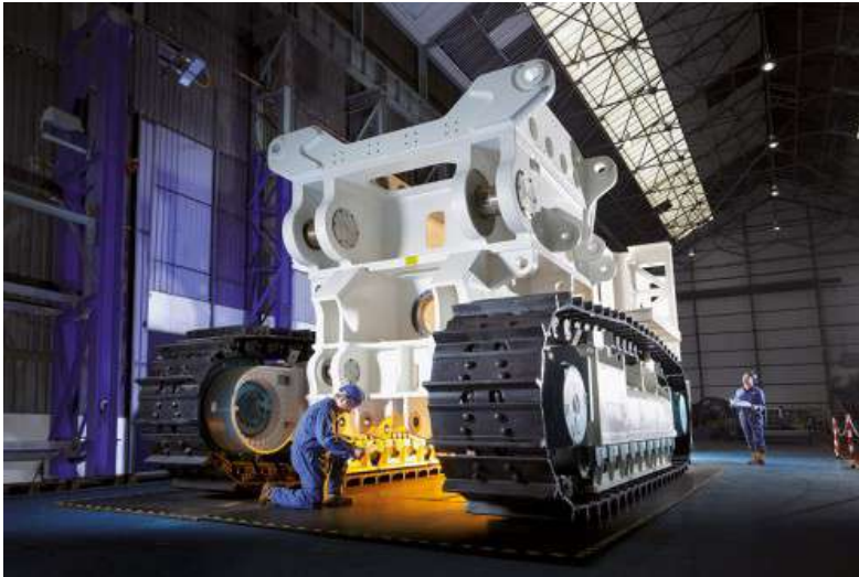
Chassis of seabed rock cutter (adapted cable trencher)
