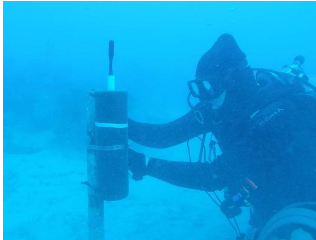
Deployment of an acoustic recorder in Florida Keys National Marine Sanctuary. NOAA
