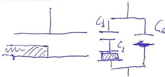
$$C = C_0 + \frac{C_1 C_2}{C_1 + C_2}$$
