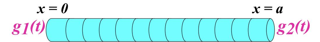
$$\frac{\partial u}{\partial t} = d\frac{\partial^2 u}{\partial x^2}, \quad 0 \le x \le a, \quad 0 \le t \le T$$
