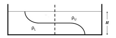
A schematic of a lock exchange experiment. In this case fluid of density  $\rho_U$  is separated by a vertical partition – the lock gate – from denser fluid with density  $\rho_L$ . Both fluids are initially at rest. When the gate is removed a dense gravity current will flow along the bottom to the right and a buoyant current will flow along the top to the left
