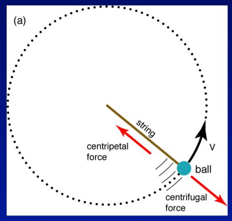
Centripetal force is the actual force that keeps the ball "tethered" (here it is the string, but it can be gravitational force)
