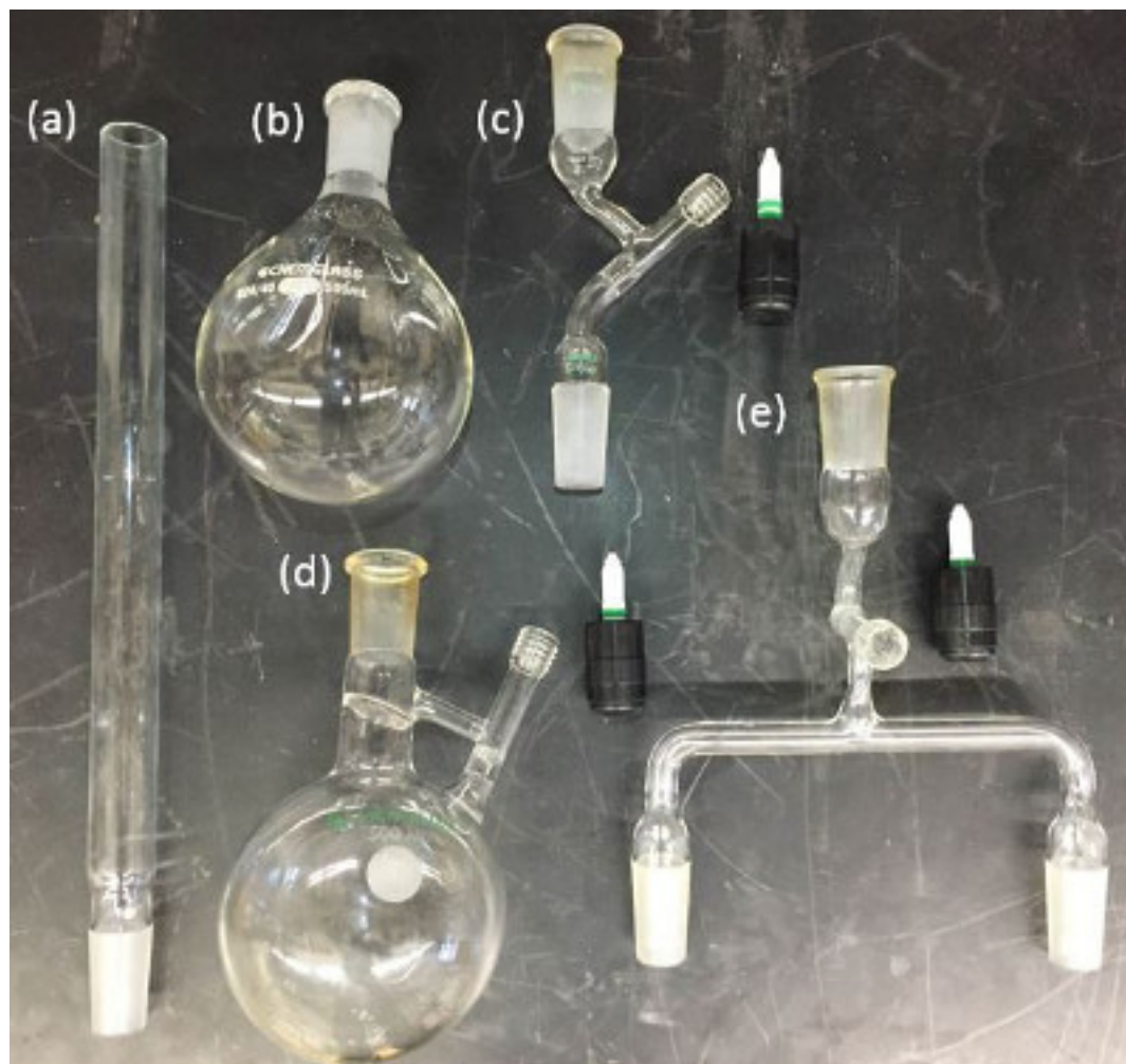
Figure 1. Glassware needed to make a ketyl pot and perform a vacuum transfer to a Straus flask. (a) Funnel for adding solvent to ketyl pot; (b) 500-mL round-bottom flask; (c) 180° adapter; (d) 500-mL Straus flask; (e) vacuum transfer bridge.
