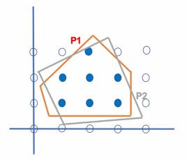
Set X composed of BLUE points. P1 and P2 are two different formulations for X.
