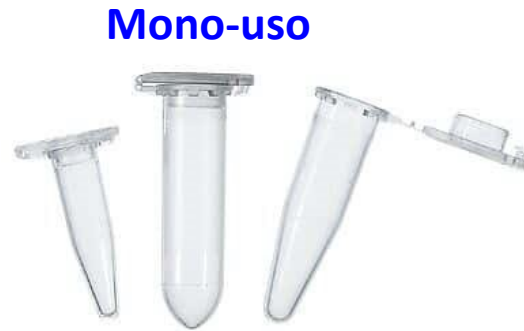
Provette "Eppendorf" (Eppendorf tube)
