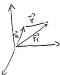
$\vec{r} = \vec{r}_1 - \vec{r}_2$  Relative separation vector; the origin is the first particle.
