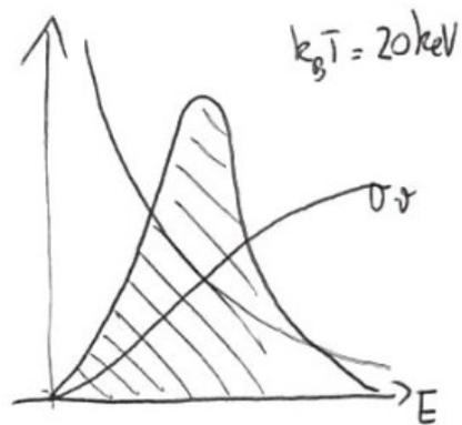
At low temperature there is a little overlap between  $n(E)$  and  $\sigma v$  and the average is small. At <sup>very</sup> high  $T$ , the area of Boltzmann distribution becomes small and again the average value of  $\sigma v$  is small.
