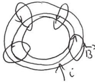
The combination of the 2 is at the basis of the so called TOKAMAK. (TORoidal NAja KAmera MAgnetische KATUShka)
