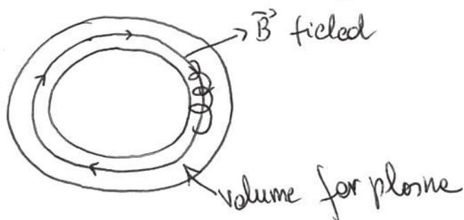
Like that there is a problem, only with a toroidal field, the problem is that the magnetic field is not constant with the radius
