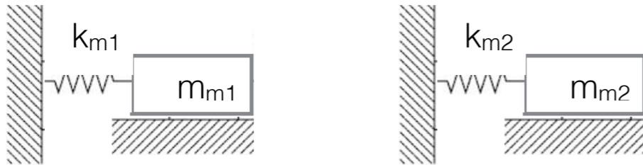
$$\begin{matrix} m_{m1} & & k_{m1} \\ \begin{bmatrix} 3 & 0 \\ 0 & 3/2 \end{bmatrix} & \begin{Bmatrix} \ddot{q}_1 \\ \ddot{q}_2 \end{Bmatrix} & + & \begin{bmatrix} 3 & 0 \\ 0 & 15/4 \end{bmatrix} & \begin{Bmatrix} q_1 \\ q_2 \end{Bmatrix} & = & \begin{Bmatrix} 0 \\ 0 \end{Bmatrix} \\ & m_{m2} & & & k_{m2} & & \end{matrix}$$
