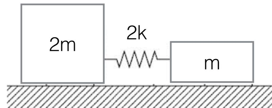
$$\begin{bmatrix} 2k - \omega_i^2 2m & -2k \\ -2k & 2k - \omega_i^2 m \end{bmatrix} \begin{Bmatrix} x_1 \\ x_2 \end{Bmatrix} = \begin{Bmatrix} 0 \\ 0 \end{Bmatrix}$$
