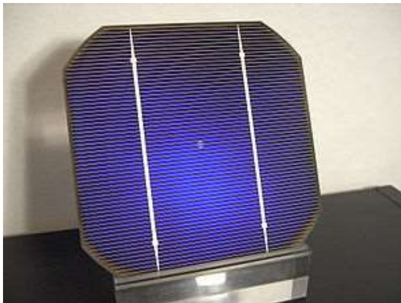
Cella in silicio monocristallino
