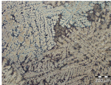
Figure 5. Microstructure of alloy Ni49.5-Ti25.5-Zr10-Nb15 (at. %), plasma
