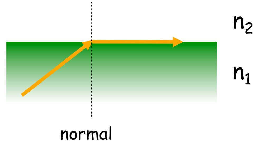
At a particular angle of incidence (**the critical angle  $\theta_c$** ) the refracted ray will travel along the boundary ie  $\theta_2 = 90^\circ$
