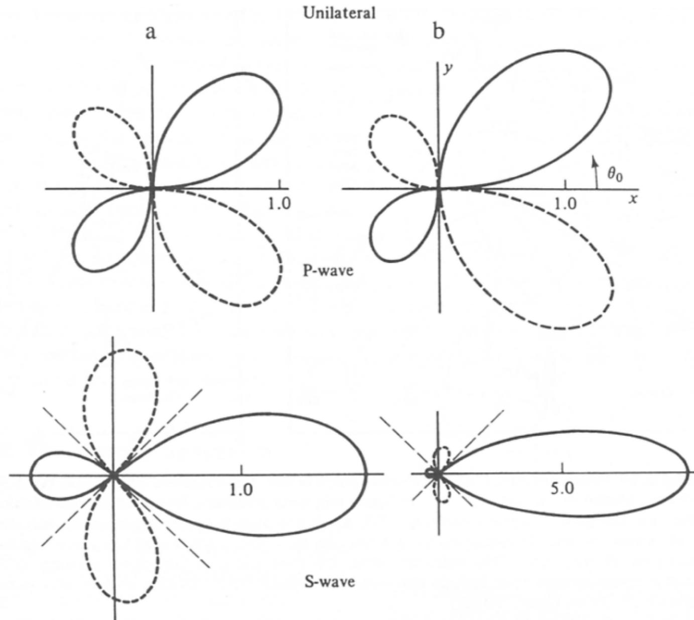
**FIGURE 9.10** The variability of *P*- and *SH*-wave amplitude for a propagating fault (from left to right). For the column on the left  $v_r/v_s = 0.5$ , while for the column on the right  $v_r/v_s = 0.9$ . Note that the effects are amplified as rupture velocity approaches the propagation velocity. (From Kasahara, 1981.)
