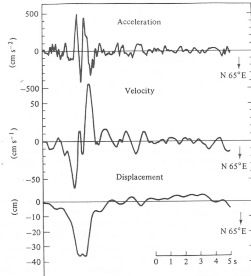
**FIGURE 9.7** A recording of the ground motion near the epicenter of an earthquake at Parkfield, California. The station is located on a node for  $P$  waves and a maximum for  $SH$ . The displacement pulse is the  $SH$  wave. Note the trapezoidal shape. (From Aki, *J. Geophys. Res.* 73, 5359–5375, 1968; © copyright by the American Geophysical Union.)
