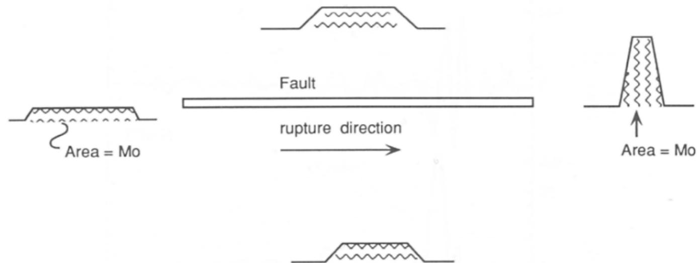
**FIGURE 9.9** Azimuthal variability of the source time function for a unilaterally rupturing fault. The duration changes, but the area of the source time function is the seismic moment and is independent of azimuth.
