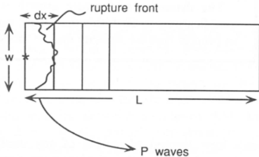
**FIGURE 9.5** Geometry of a one-dimensional fault of width  $w$  and length  $L$ . The individual segments of the fault are of length  $dx$ , and the moment of a segment is  $m dx$ . The fault ruptures with velocity  $v_r$ .
