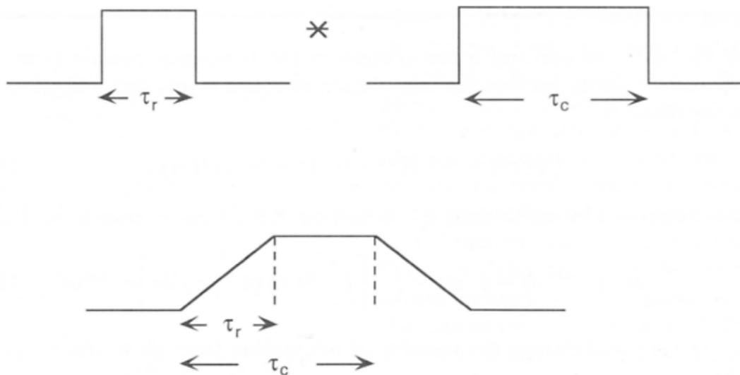
**FIGURE 9.6** The convolution of two boxcars, one of length  $\tau_r$  and the other of length  $\tau_c$  ( $\tau_c > \tau_r$ ). The result is a trapezoid with a rise time of  $\tau_r$ , a top of length  $\tau_c - \tau_r$ , and a fall of width  $\tau_r$ .
