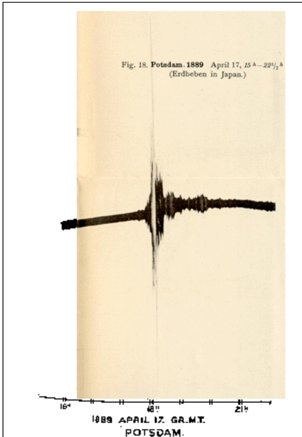
This seismogram was recorded in Potsdam in 1889, for a Japanese earthquake, with von Rebeur's horizontal pendulum.
