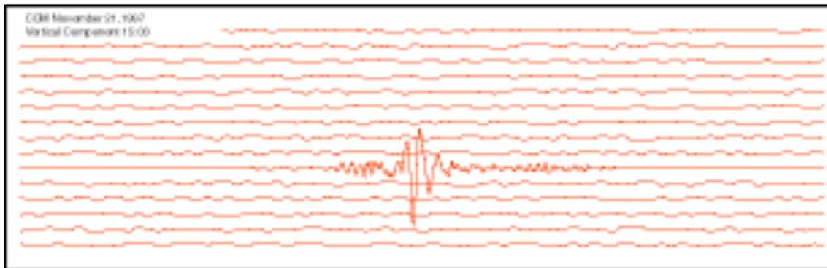
For most of the last century, seismograms were recorded on sheet of paper, either with ink or photographically. We call such records "analog" records to distinguish them from digital recordings. These records are read just like a book - from top-to-bottom and left-to-right.
