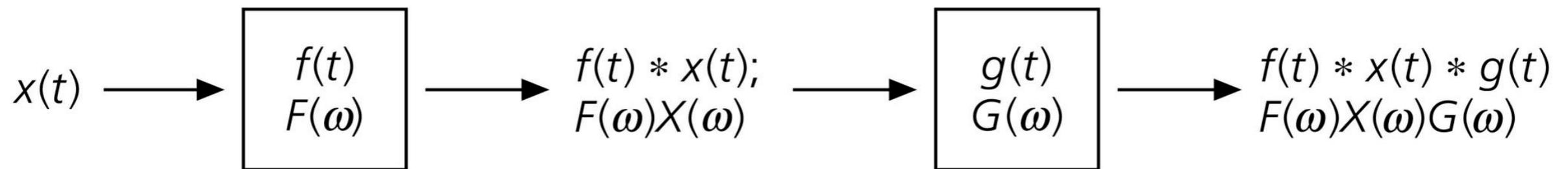
The output of a linear system is the convolution of the input and the impulse response (Green's function)
