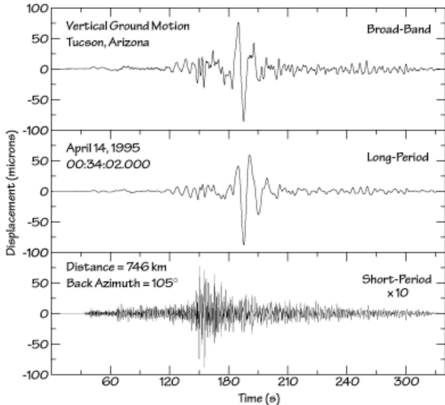
Top panel shows the vibrations measured using a **broad-band** seismometer, the middle panel shows the vibrations as they would be detected by the long-period sensor, and the bottom panel the vibrations that would be sensed by a **short-period** sensor (scaled by a factor of 10). The displacements are shown in microns, which are  $1 \times 10^{-6}$  m.
