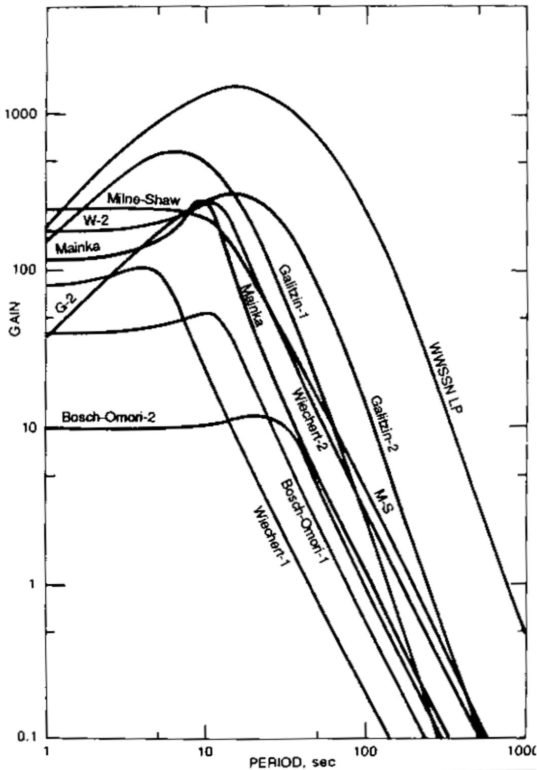
**Instrument response curves** for a suite of classic seismometers, indicating their magnification as a function of period. For very long periods (low frequencies) all of the curves fall as  $1/T^2$ , being sensitive to ground acceleration; for shorter periods the pendulum-type behaviour is sensitive to displacement.
