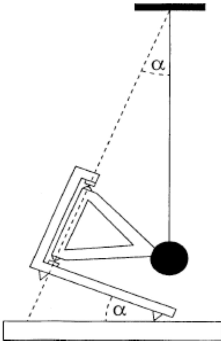
In the "garden-gate" pendulum the mass moves in a nearly horizontal plane around a nearly vertical axis. The restoring force is now  $g(\sin\alpha)$  where  $\alpha$  is the angle between the vertical and the rotation axis.
