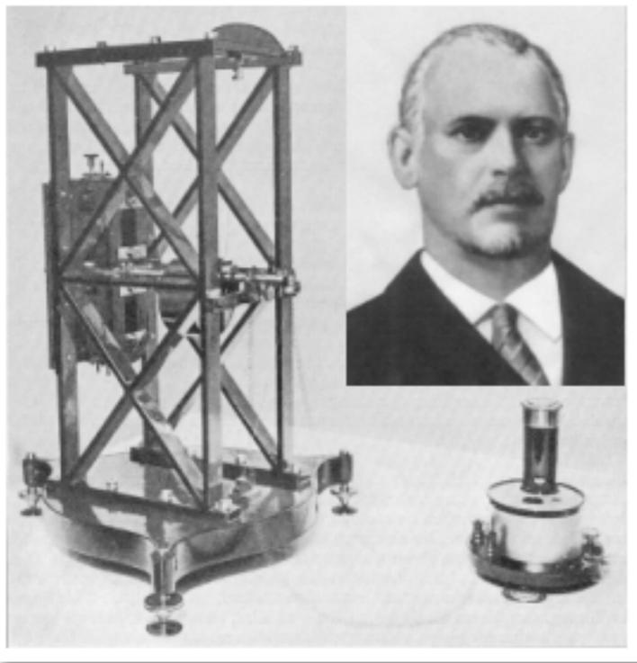
In 1906 Boris Galitzin designed a seismograph that made the need for mechanical linkage between the pendulum and the recorder obsolete. Instead he mounted a coil of wire on the pendulum and suspended both between the poles of a magnet that was fixed to the earth. During an earthquake, the magnetic field was moved around a coil generating electrical current. Because of this the recorder could now be separated from the seismograph by use of a wire.
