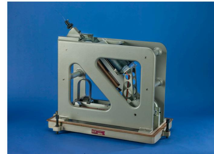
3 short period, 1s pendulum and 0.7s galvanometer periods, and 3 long-period, 15s pendulum and 100s galvanometer periods, instruments were deployed, starting from the 1960s, as a global array to record horizontal and vertical motion. The recordings, with accurate timing and standard response, have been extensively utilized because the original photographic records were filmed and distributed to data centers .
