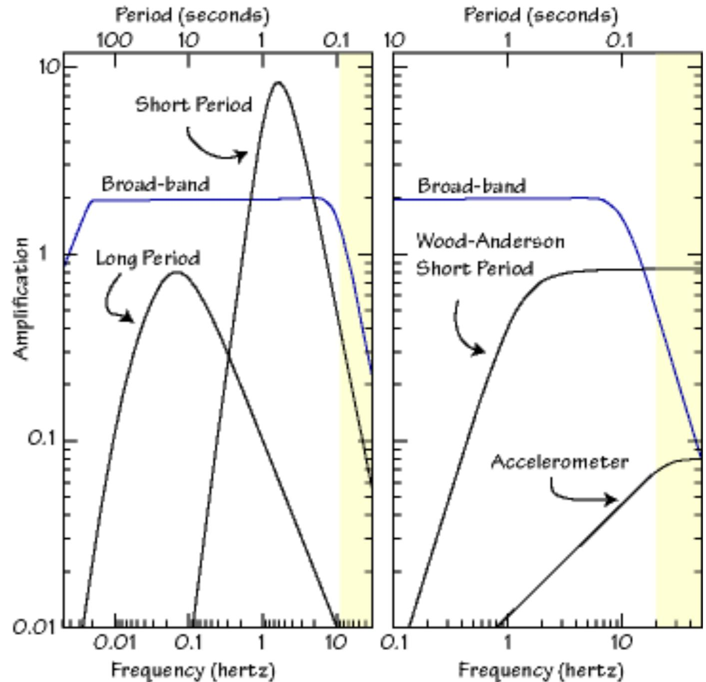
The broad band instrument senses most frequencies equally well; the long-period and short period instruments are called "narrow" band, because they preferentially sense frequencies near 1/(15 s) and 1 hertz respectively. The yellow region is the low end of the frequency range audible to most humans (we can hear waves around 20 hertz to 20,000 hertz).
