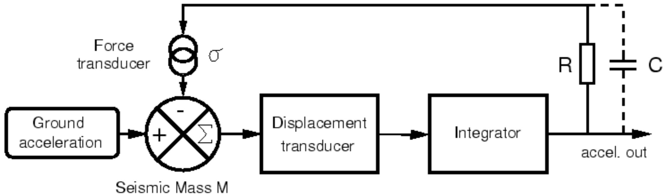
circuit of a force-balance accelerometer (FBA), widely used for earthquake **strong-motion** recording
