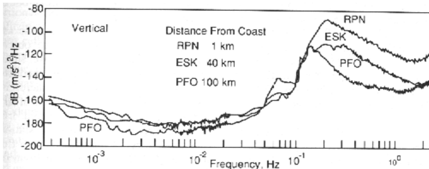
Observed seismic noise as a function of frequency (power spectrum). Note the peak at 0.2 Hz and decrease with distance from the coast.
