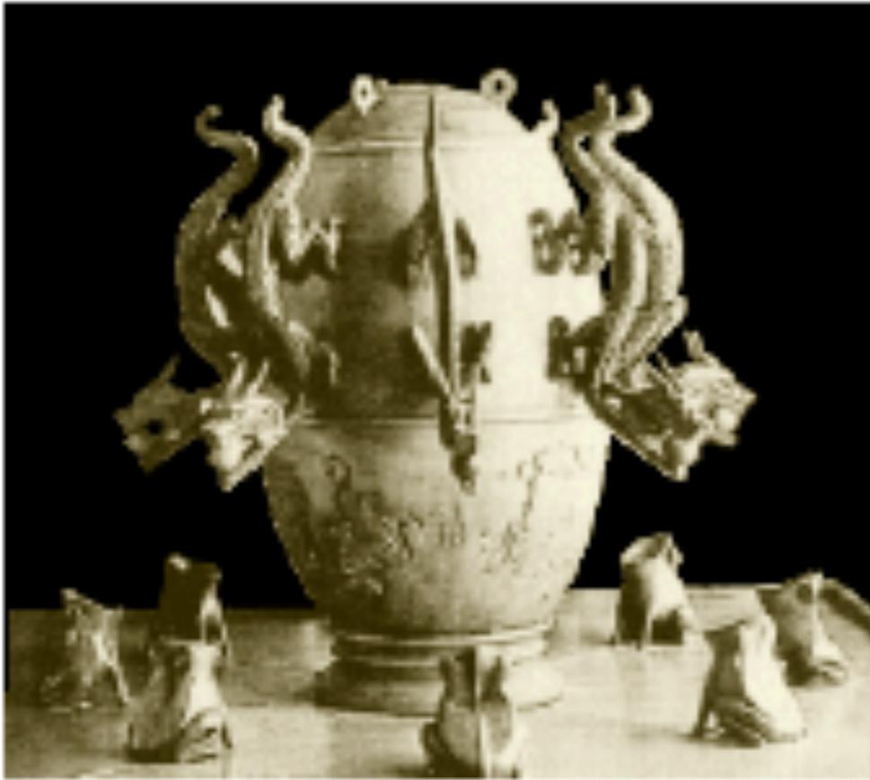
Chang Heng's quaint device can technically be called a **seismoscope**, an instrument that primarily measures the direction of ground motion, without necessarily noting time or amplitude.
