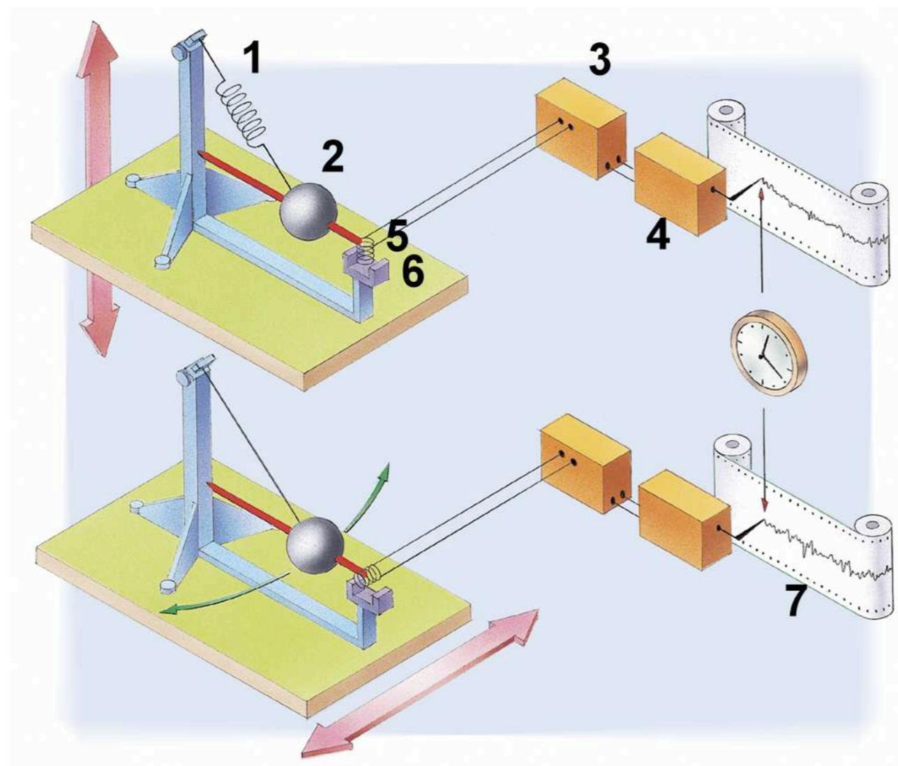
The first seismographs were built in the late 19th Century. They were a mechanical synthesis of sorts - a seismometer rigged up to transfer its motions to some kind of timekeeping and recording device.
