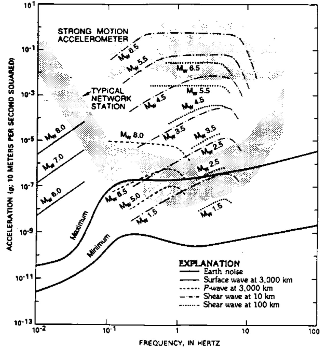
Comparison of accelerometer and regional-network recording capabilities relative to average noise level and ground accelerations caused by various size events at different distances.
