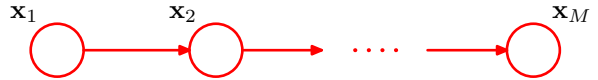
Figure 8.10 This chain of M discrete nodes, each having K states, requires the specification of K - 1 + (M - 1)K(K - 1) parameters, which grows linearly with the length M of the chain. In contrast, a fully connected graph of M nodes would have K^M - 1 parameters, which grows exponentially with M .
