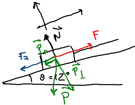
$$\begin{aligned} & \perp \left\{ \begin{array}{l} \vec{N} + \vec{P}_{\perp} = 0 \\ \vec{F} + \vec{F}_f + \vec{P}_{\parallel} = m\vec{a} = 0 \end{array} \right. \rightarrow N = P_{\perp} = mg \cos \theta \\ & \parallel \end{aligned}$$
