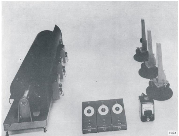
**Short period (on the left) and long period (on the right) seismograph recording instruments**
