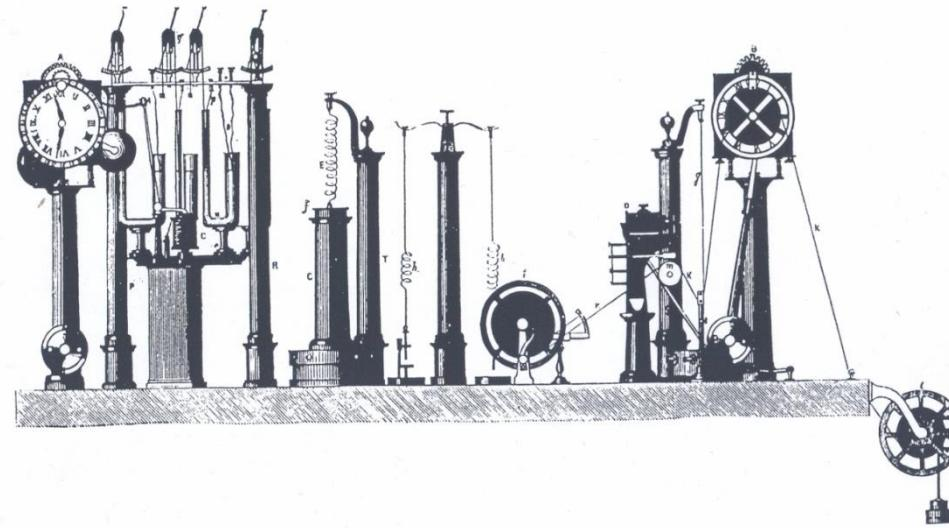
FIG. 4. Palmieri's "sismografo elettro-magnetico" (reproduced from *The Engineer*, 33, 1877, p. 407). Vertical motion is detected by a mass on a spiral spring *E*. The U-tubes *n* detect horizontal motion. Paper is unrolled from the drum *i* and a pencil mark put on the paper at *m*. The speed of the paper is regulated by the clock *B*. The clock *A* is stopped by the earthquake to give the time of the shock.
