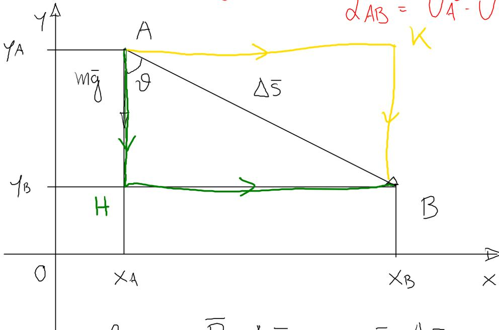
$$\begin{aligned} \Delta U_{AB} &= \vec{P} \cdot \Delta \vec{S} = m\vec{g} \cdot \Delta \vec{S} = mgy \Delta S \cos \vartheta \\ &= mgy (y_A - y_B) \end{aligned}$$
