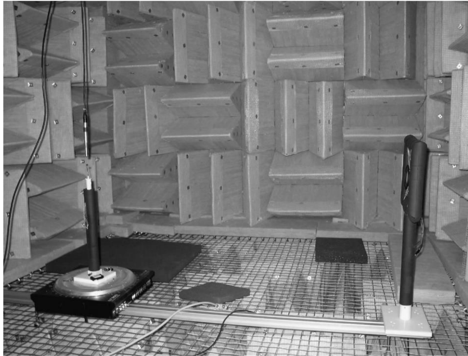
Figure 3.17 Setup in an anechoic chamber for measurement of a microphone's directivity
