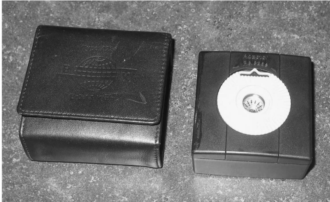
Figure 3.16 Sound source for measurement of a microphone's sensitivity
