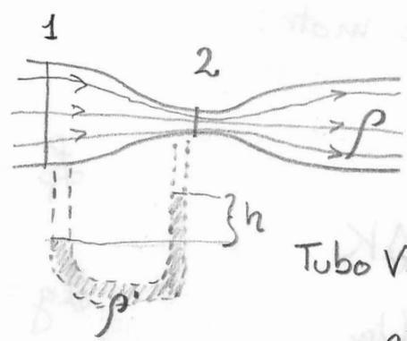
$$v_2 = v_1 \frac{S_1}{S_2} > v_1$$
