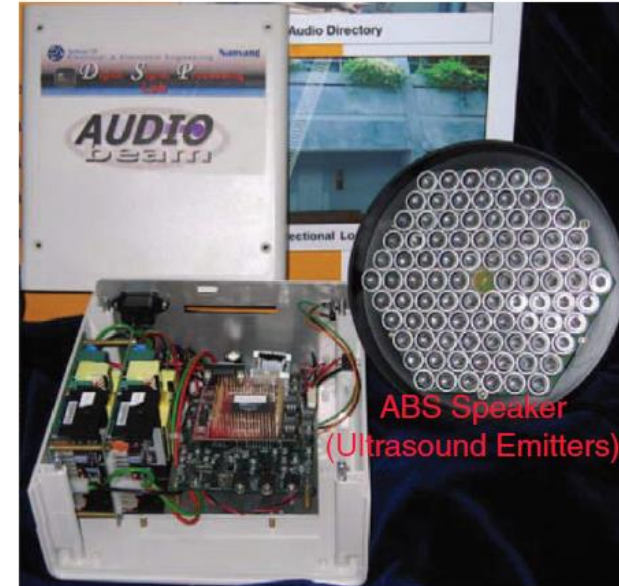
Fig. 6 ABS and its ultrasound emitters.
