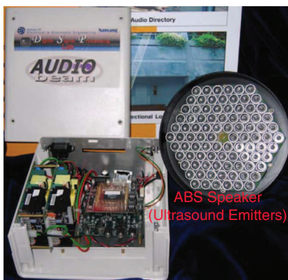
Fig. 6 ABS and its ultrasound emitters.
