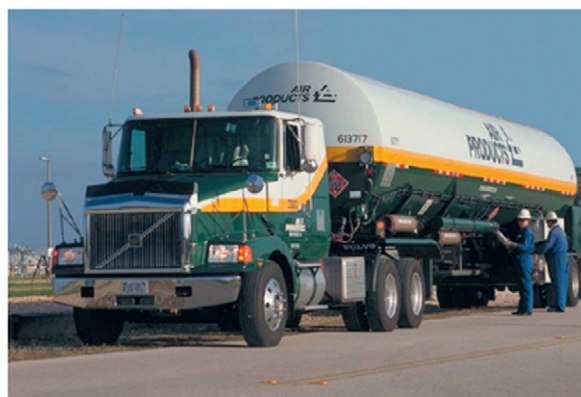
Figure 12 Tube tanker for \text{LH}_2 transport. Courtesy of Air Products.
