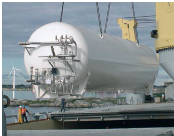
Figure 13 Transportable dewar for bulk LH 2 transport (capacity 300 N m 3 ). Courtesy of Linde Kryotechnik AG.
