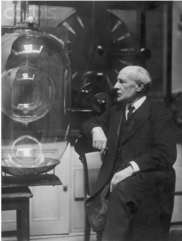
Figure 1 Sir James Dewar, FRS, 1842–1923, beside his vacuum-insulated, double-walled, silvered-glass, experimental apparatus developed for his pioneering work in hydrogen liquefaction.
