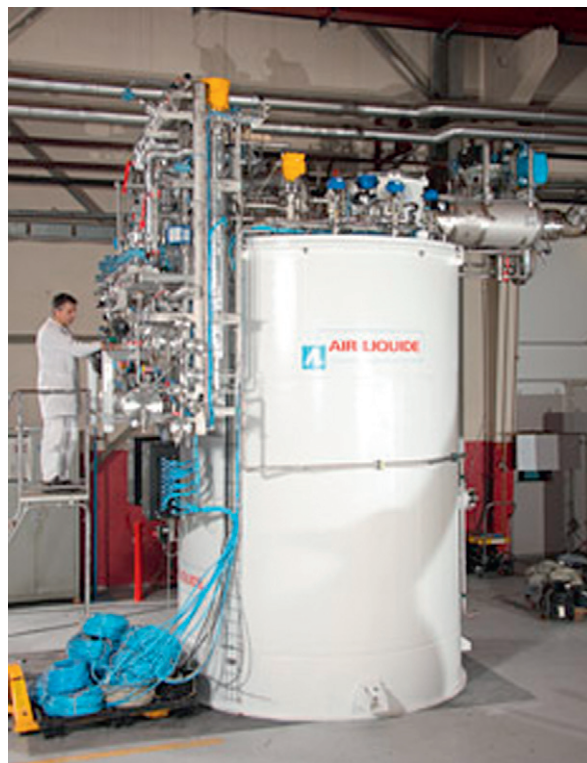
Figure 9 Small- to medium-scale hydrogen liquefier. Courtesy of Air Liquide.
