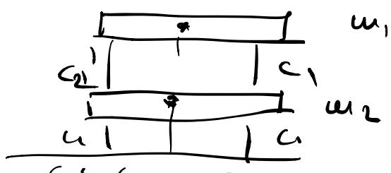
$$\left\{ \begin{array}{l} -c_2 x_1 - c_1 x_1 + c_1 x_2 = u_1 \\ -c_2 x_2 - c_1 x_2 + c_1 x_1 = u_2 \end{array} \right.$$
