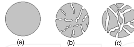
Figure 5. Schematic presentation of different matrix types (a) non-porous beads (b) microporous beads (c) macroporous beads
