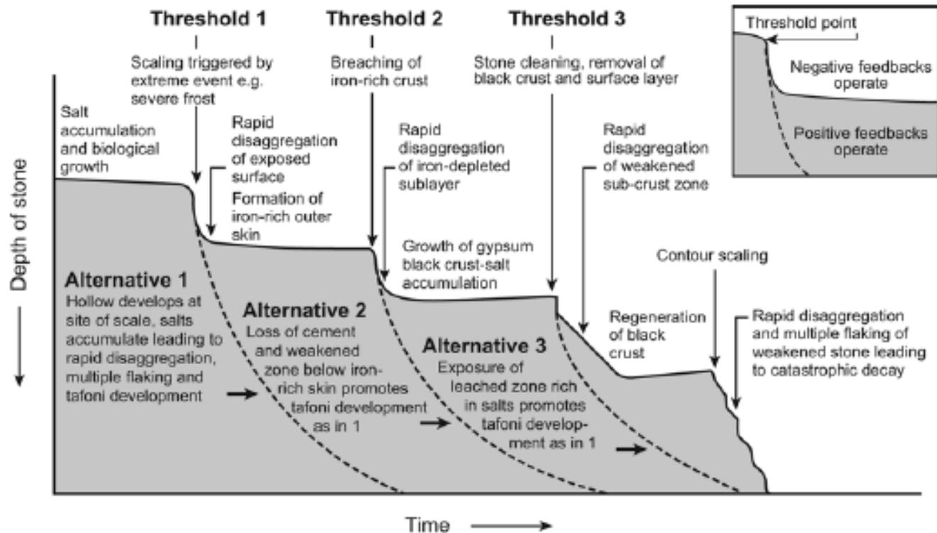
**Figure 3** Hypothetical decay pathways for quartz sandstone used as a building material in a polluted environment. The inset identifies feedback options at critical thresholds of decay associated with rapid surface loss of material
