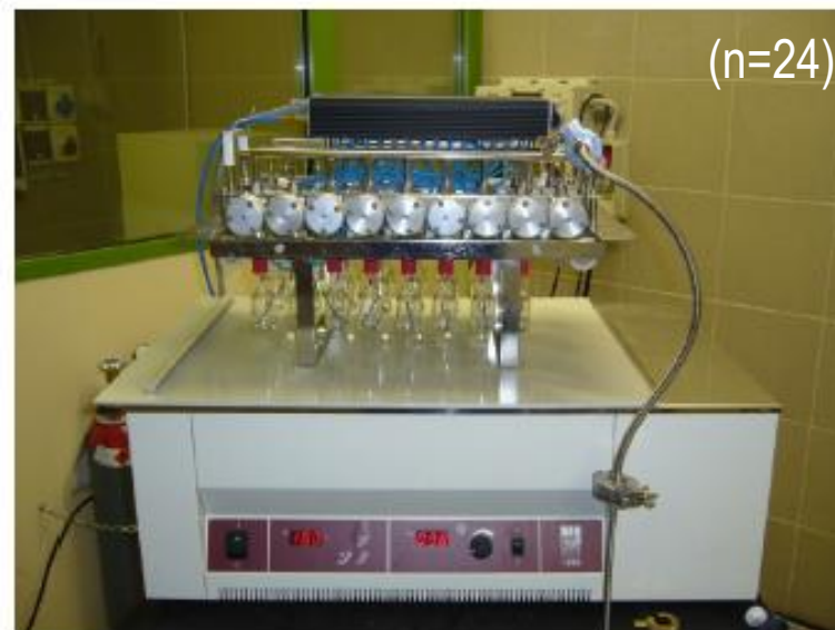
Schema del Thermo Finnigan HDO equilibrator device
