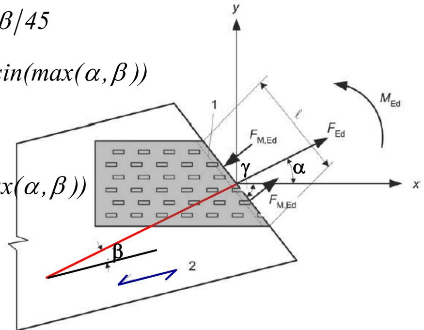
$$f_{a,\alpha,0,d} = \max \begin{cases} f_{a,0,0,d} + k_1 \alpha & \alpha \leq \alpha_0 \\ f_{a,0,0,d} + k_1 \alpha_0 + k_2 (\alpha - \alpha_0) & \alpha_0 < \alpha \leq 90^\circ \end{cases} \begin{cases} k_1 \\ k_2 \end{cases} \text{ sperimentalmente}$$
