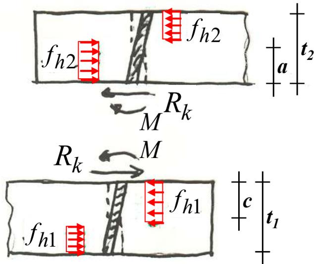
$$\begin{cases} R_k = f_{h,2,k} \cdot d \cdot (2a - t_2) \\ M = f_{h,2,k} \cdot d \cdot \left[ \frac{a^2}{2} - (t_2 - a) \left( a + \frac{t_2 - a}{2} \right) \right] \\ M = f_{h,1,k} \cdot d \cdot \left[ \frac{c^2}{2} - (t_1 - c) \left( c + \frac{t_1 - c}{2} \right) \right] \\ R_k = f_{h,1,k} \cdot d \cdot (2c - t_1) \end{cases}$$
