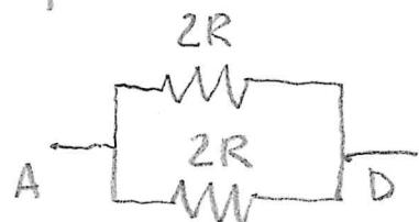
$$\frac{1}{R_{AD}} = \frac{1}{2R} + \frac{1}{2R} = \frac{1}{R} \quad R_{AD} = R = \begin{cases} A & 3\Omega \\ B & 5\Omega \end{cases}$$
